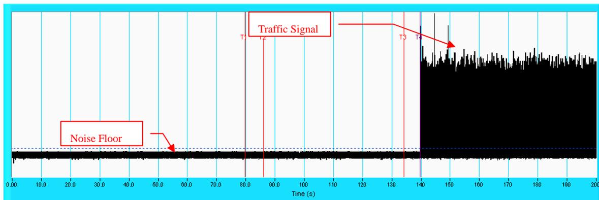
**NOTE:** T1 denotes the end of power-up time period is 80 second. T4 denotes the end of Channel Availability Check time is 140 second. Channel Availability Check time is equal to ( T4 – T1) 60 seconds.
