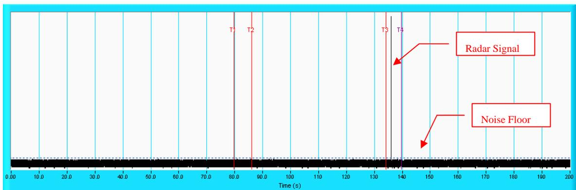
**NOTE:** T1 denotes the end of power up time period is 80 second. T3 denotes 134 second and radar burst was commenced within 54<sup>th</sup> second to 60<sup>th</sup> second window starting from the end of power-up sequence. T4 denotes the 140 second.
