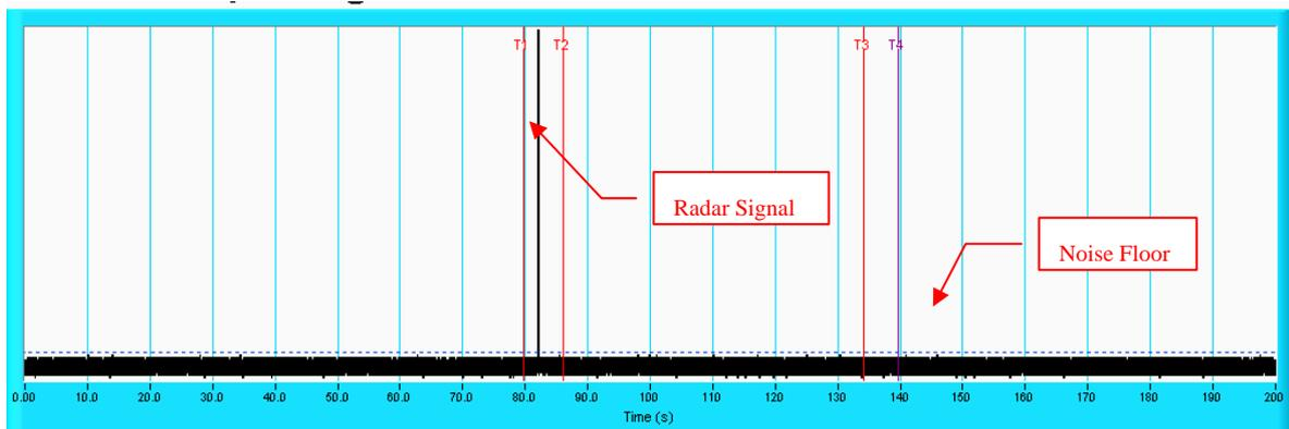
**NOTE:** T1 denotes the end of power up time period is 80 second. T2 denotes 86 second , the radar burst was commenced within a 6 second window starting from the end of power-up sequence. T4 denotes the 140 second.
