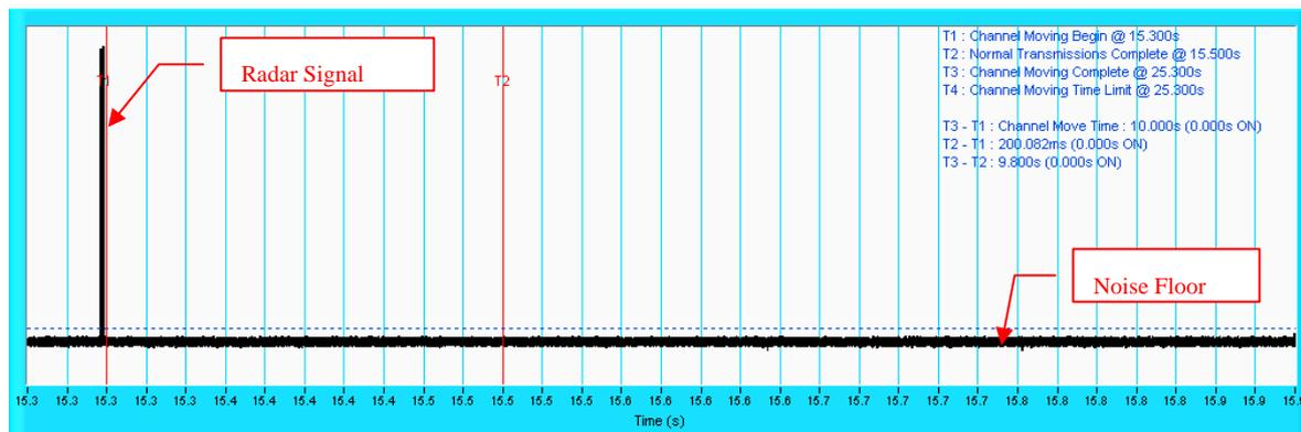
**NOTE:** An expanded plot for the device vacates the channel in the required 600ms
