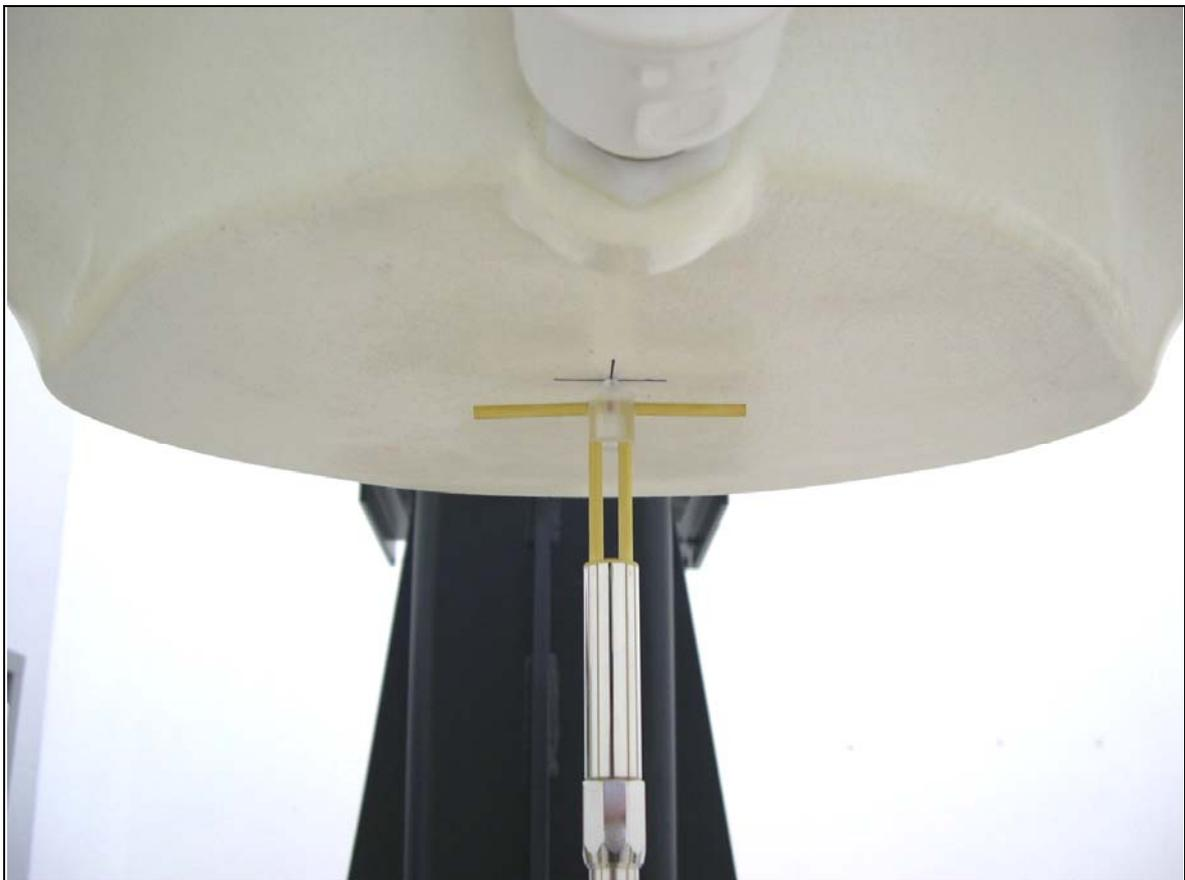
**Fig 8.2 Dipole Setup**
