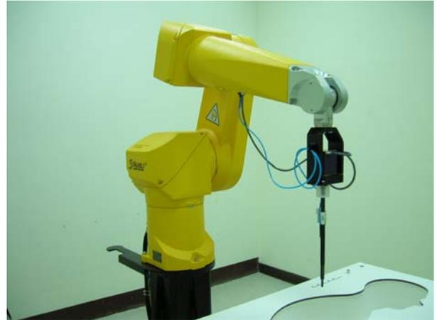
Fig. 5.2 Probe setup on robot
