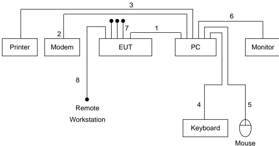
1. The RJ45 cable is connected from PC to the EUT.
