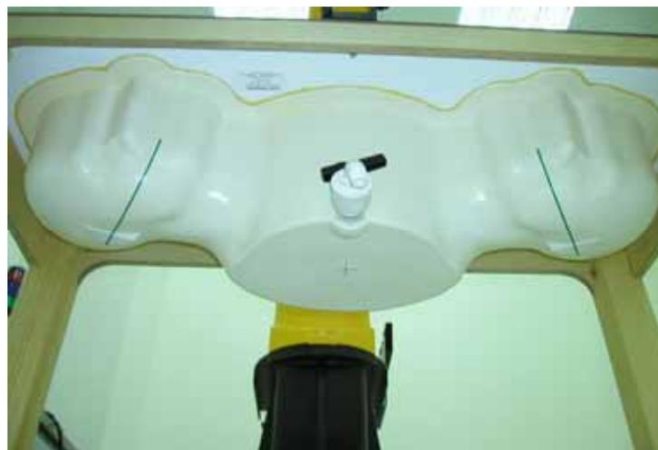
**Fig. 5.4 Bottom view of twin phantom**
