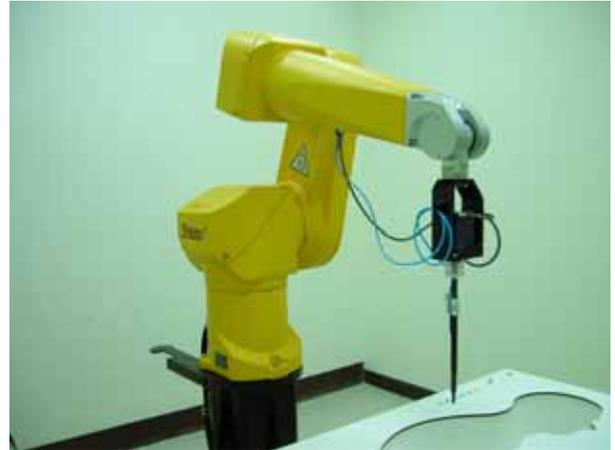
**Fig. 5.2 Probe setup on robot**
