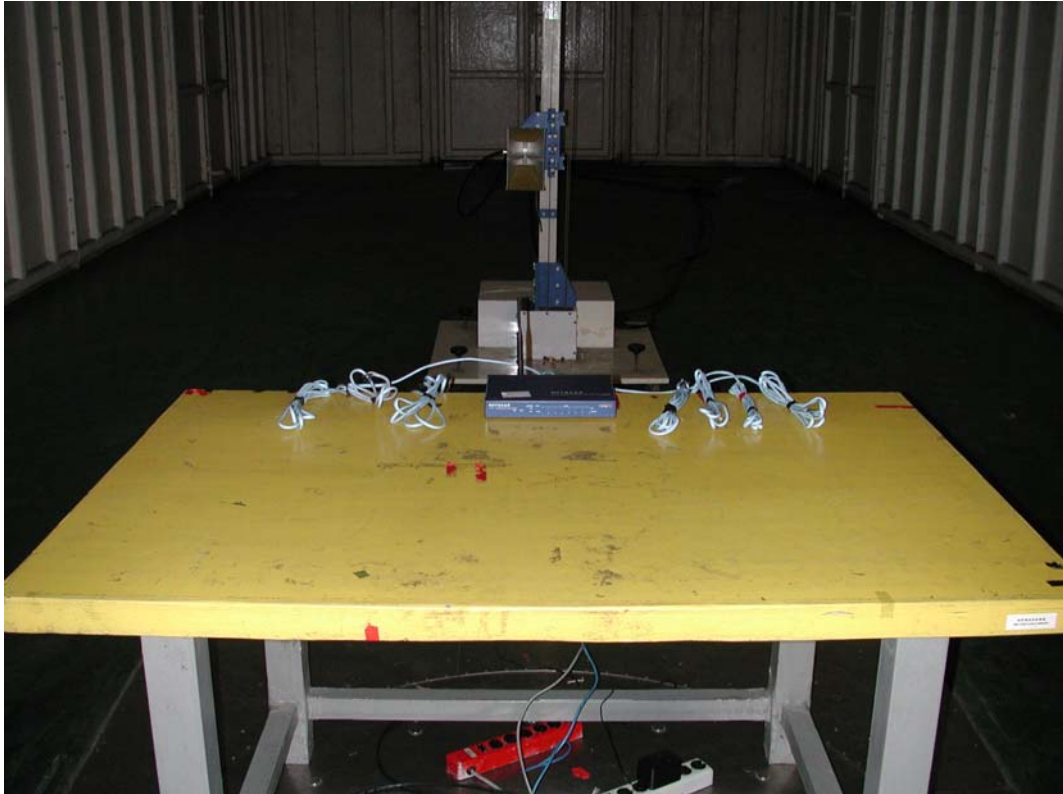
Front View of High Frequency Radiated Test
