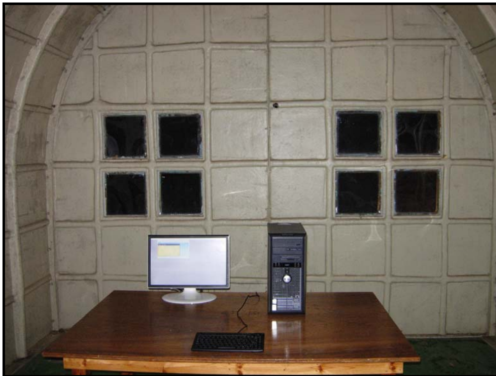
Photograph 2: Setup for Radiated Emissions
