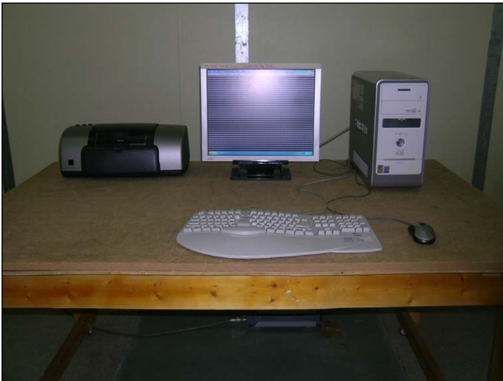
Photograph 1: Setup for Conducted Emissions
