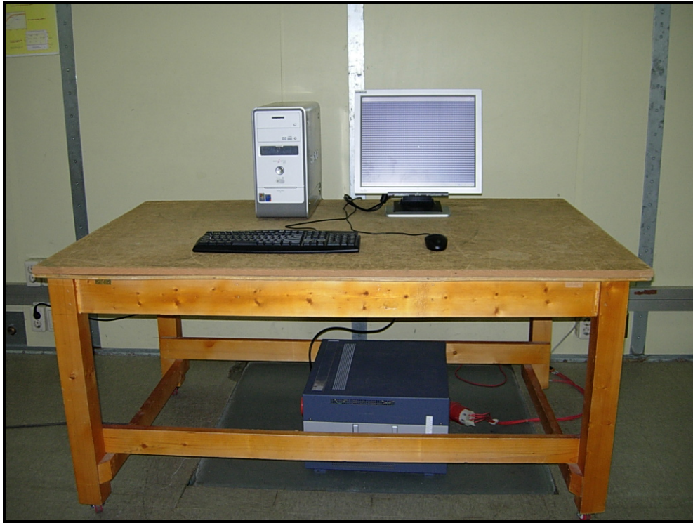
Photograph 1: Setup for Conducted Emissions
