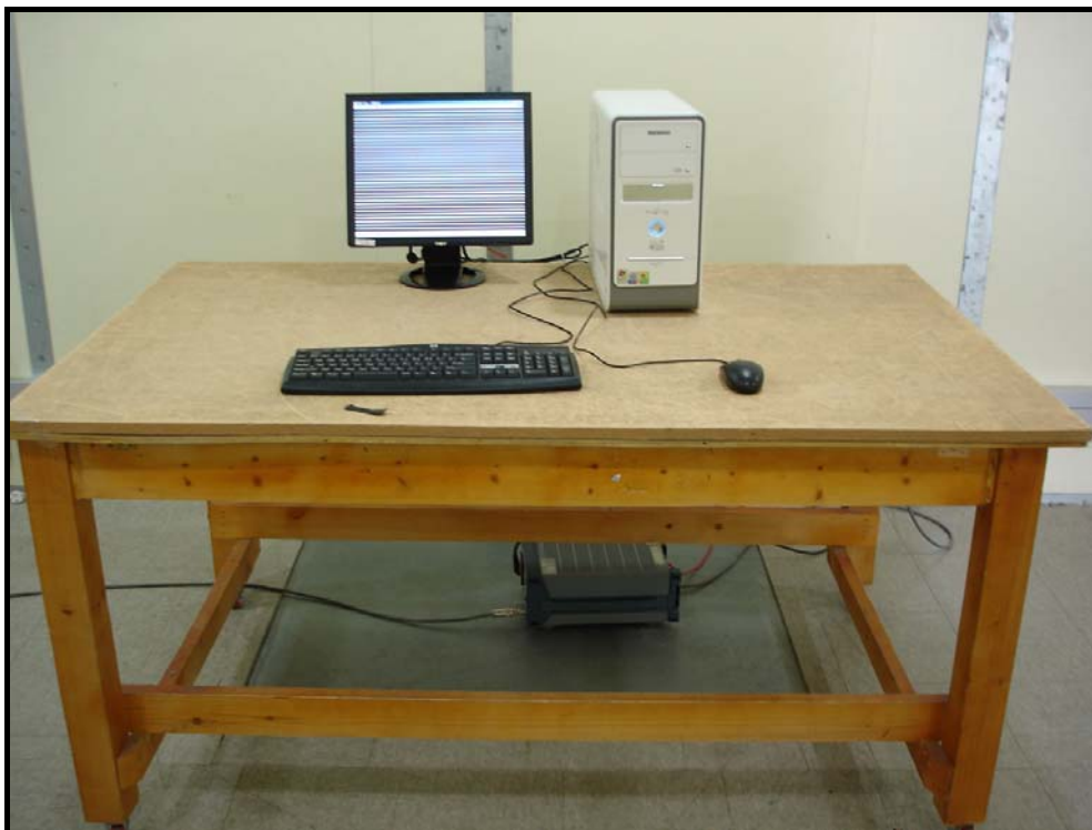
Photograph 1: Setup for Conducted Emissions
