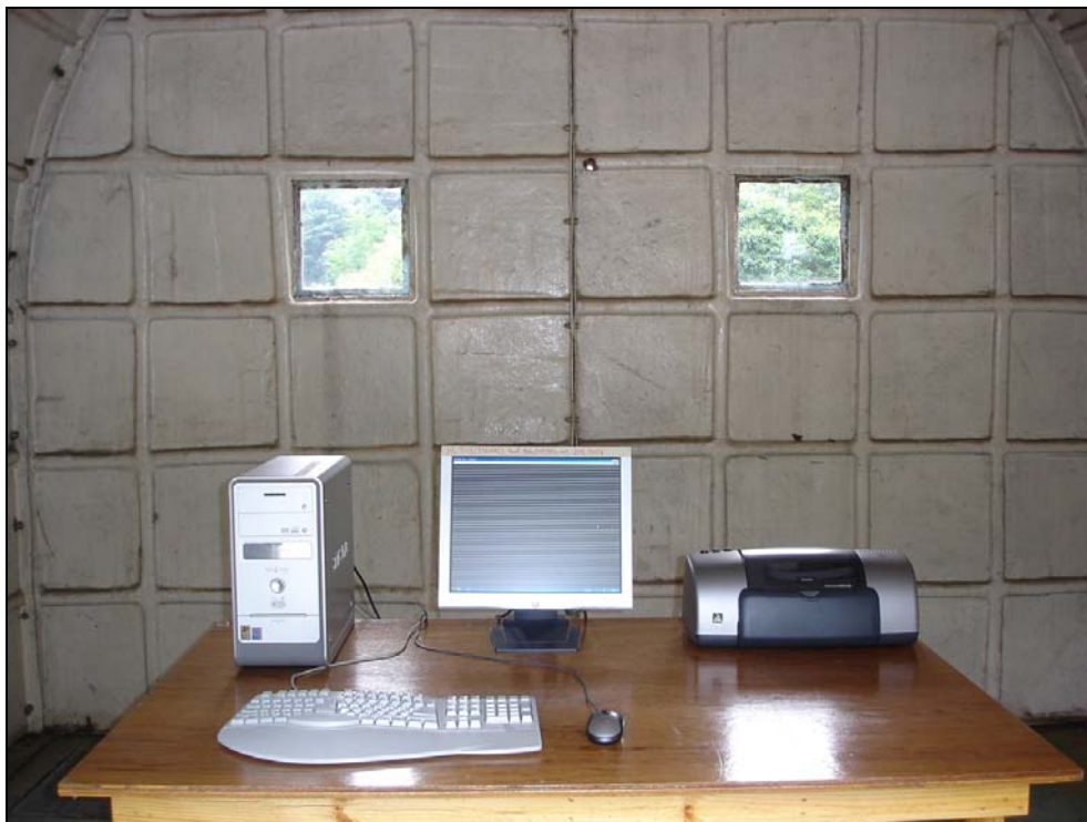
Photograph 2: Setup for Radiated Emissions
