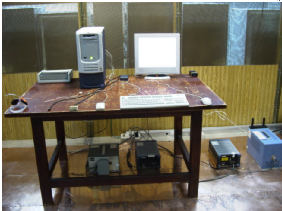
Conducted Emissions 150kHz - 30 MHz
