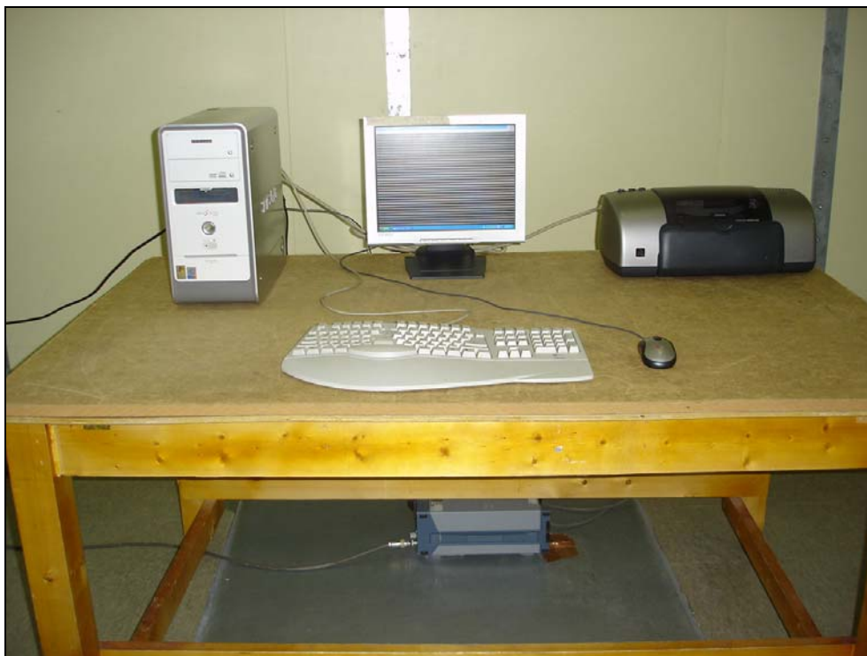
Photograph 1: Setup for Conducted Emissions
