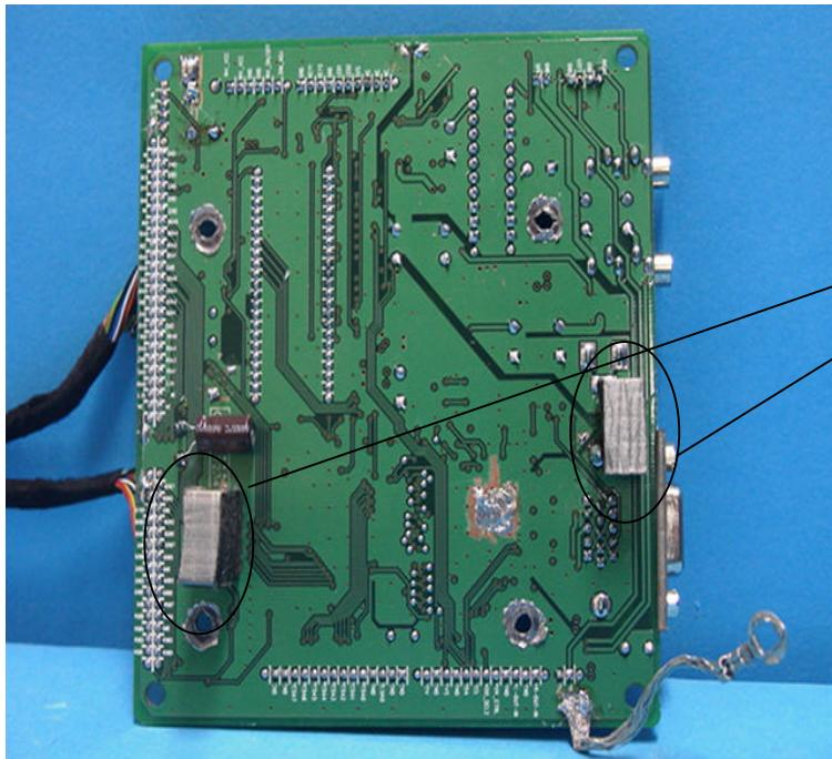
2 gaskets on the back side of AD board
