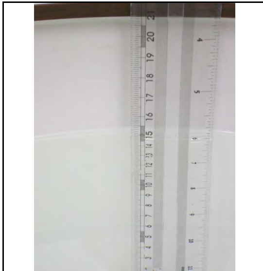
Figure 6. Liquid Height for Body SAR
