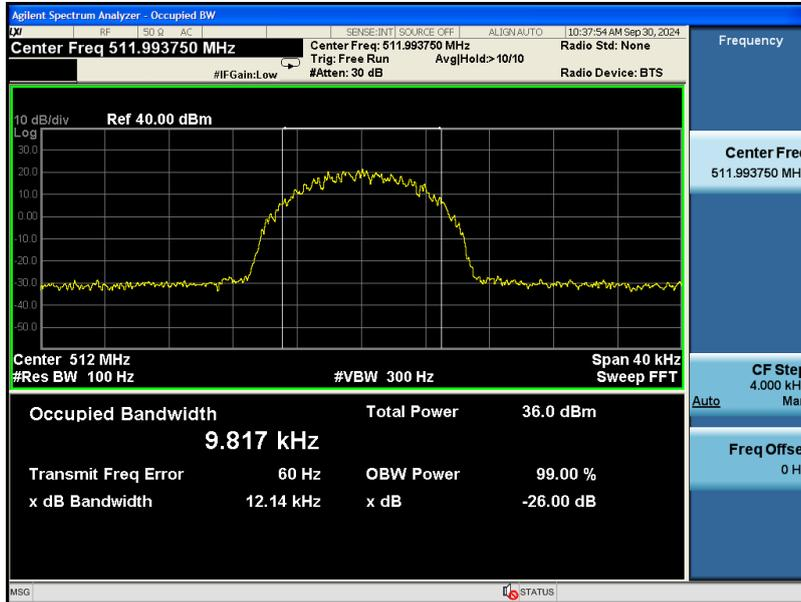
DL\_H-DQPSK\_HCH\_Output\_3dB above AGC
