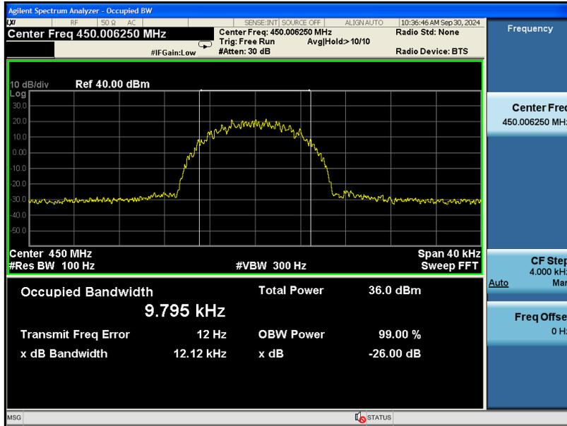
DL\_H-DQPSK\_LCH\_Output\_3dB above AGC
