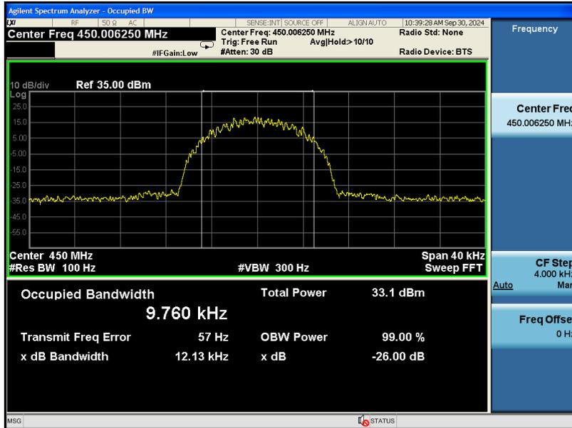
UL\_H-DQPSK\_LCH\_Output\_3dB above AGC
