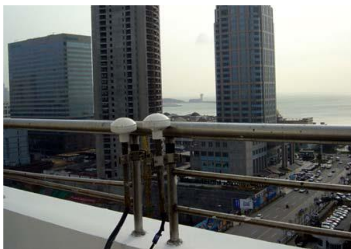
Figure 3-32Antenna spacing is too close
