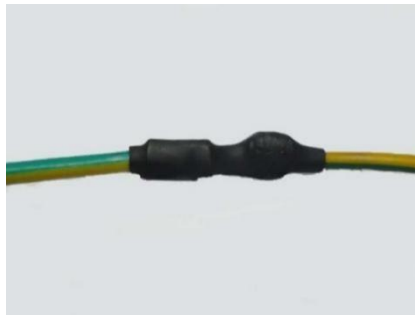
Figure 3-15 Heat shrinkable tube protection
