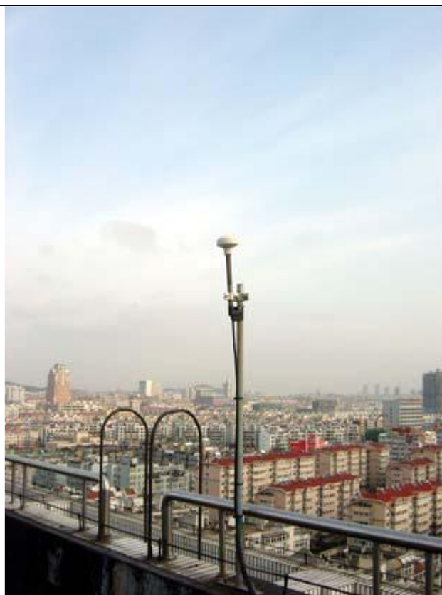
Figure 3-31Antenna position too high
