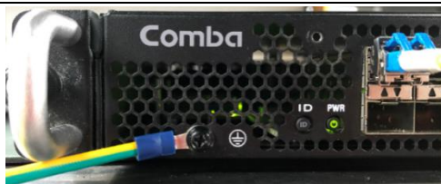
Figure 3-17 Installation diagram of AU chassis grounding wire
