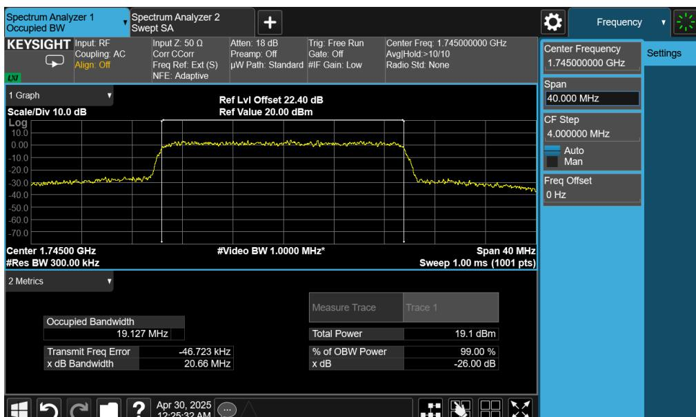
**UL\_100MHz AWGN\_MCH\_Output\_3dB above AGC**
