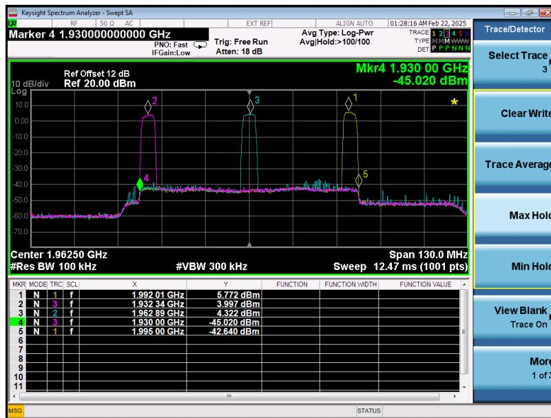
$f_0=1932.34\text{MHz}$ ,  $1962.89\text{MHz}$ ,  $1992.01\text{MHz}$  for lowest, middle, highest passband
