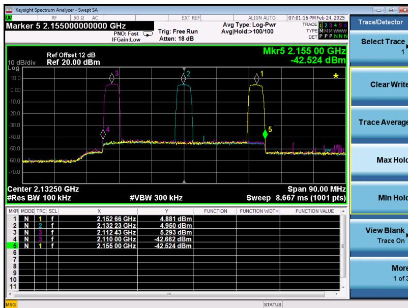
$f_0=2112.43\text{MHz}$ ,  $2132.23\text{MHz}$ ,  $2152.66\text{MHz}$  for lowest, middle, highest passband
