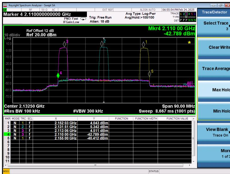
$f_0=2113.06\text{MHz}$ ,  $2131.51\text{MHz}$ ,  $2152.03\text{MHz}$  for lowest, middle, highest passband
