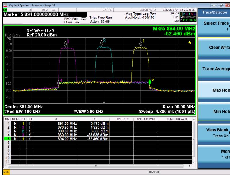
$f_0=870.90\text{MHz}$ ,  $880.80\text{MHz}$ ,  $891.55\text{MHz}$  for lowest, middle, highest passband
