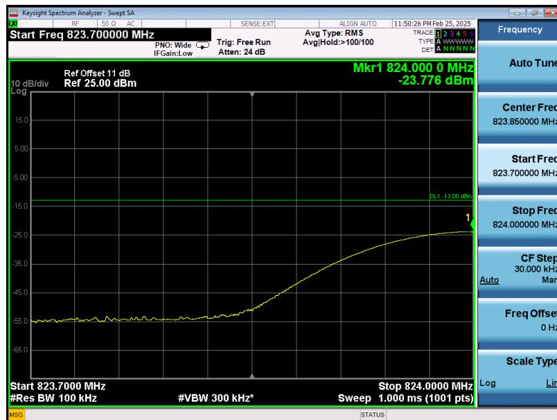
**UL\_1.25MHz AWGN input\_Lower band edge\_10dB above AGC**
