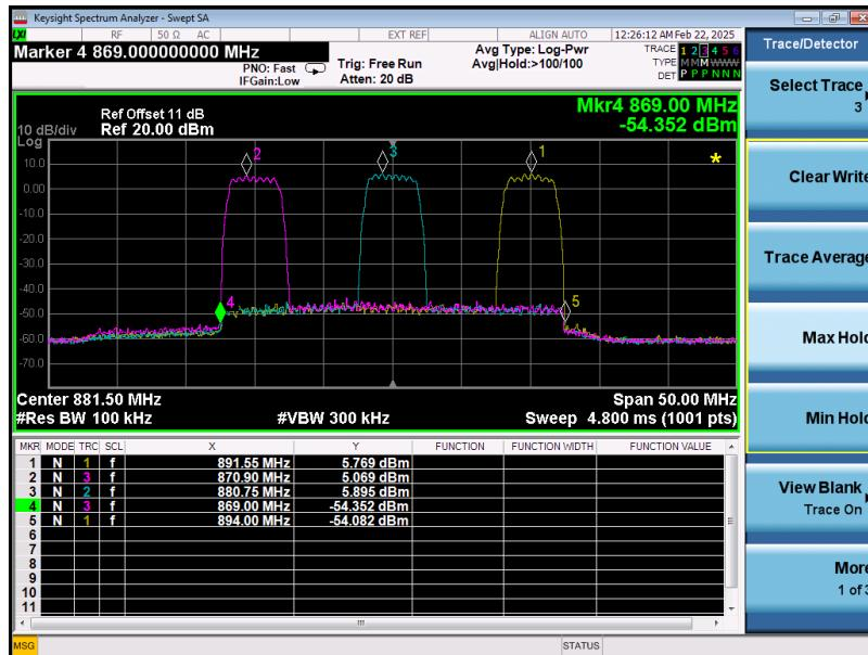
$f_0=870.90\text{MHz}$ ,  $880.75\text{MHz}$ ,  $891.55\text{MHz}$  for lowest, middle, highest passband
