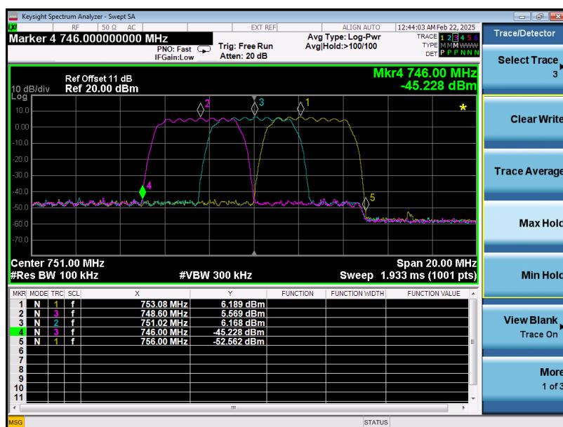
$f_0=748.60\text{MHz}, 751.02\text{MHz}, 753.08\text{MHz}$  for lowest, middle, highest passband
