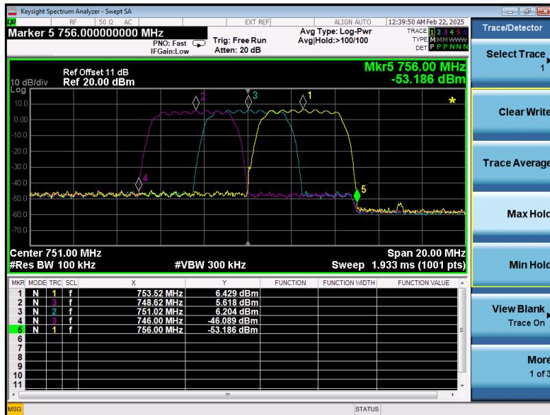
$f_0=748.62\text{MHz}$ ,  $751.02\text{MHz}$ ,  $753.52\text{MHz}$  for lowest, middle, highest passband
