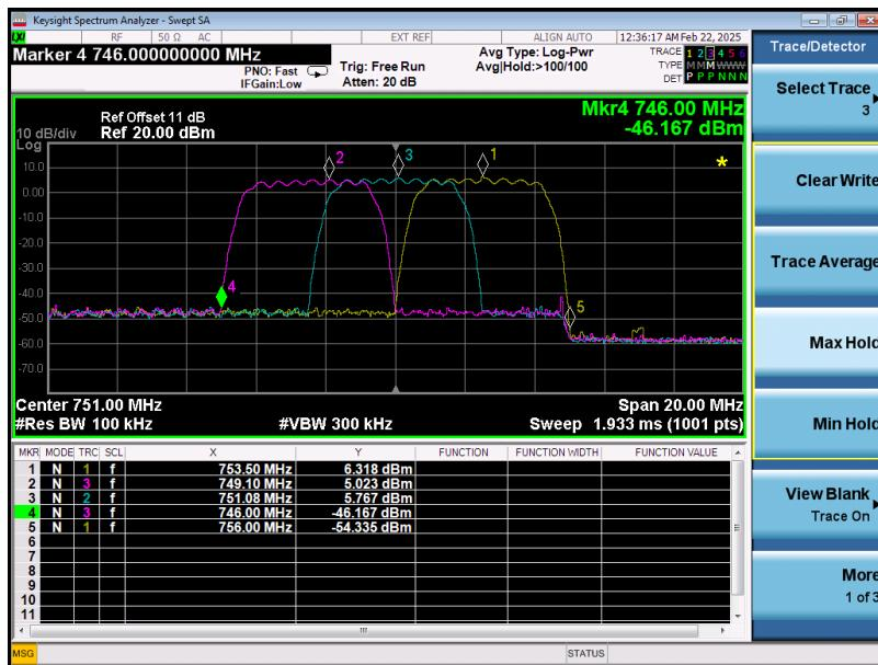
$f_0=749.10\text{MHz}$ ,  $751.08\text{MHz}$ ,  $753.50\text{MHz}$  for lowest, middle, highest passband
