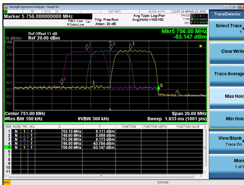
$f_0=748.60\text{MHz}, 751.08\text{MHz}, 753.10\text{MHz}$  for lowest, middle, highest passband
