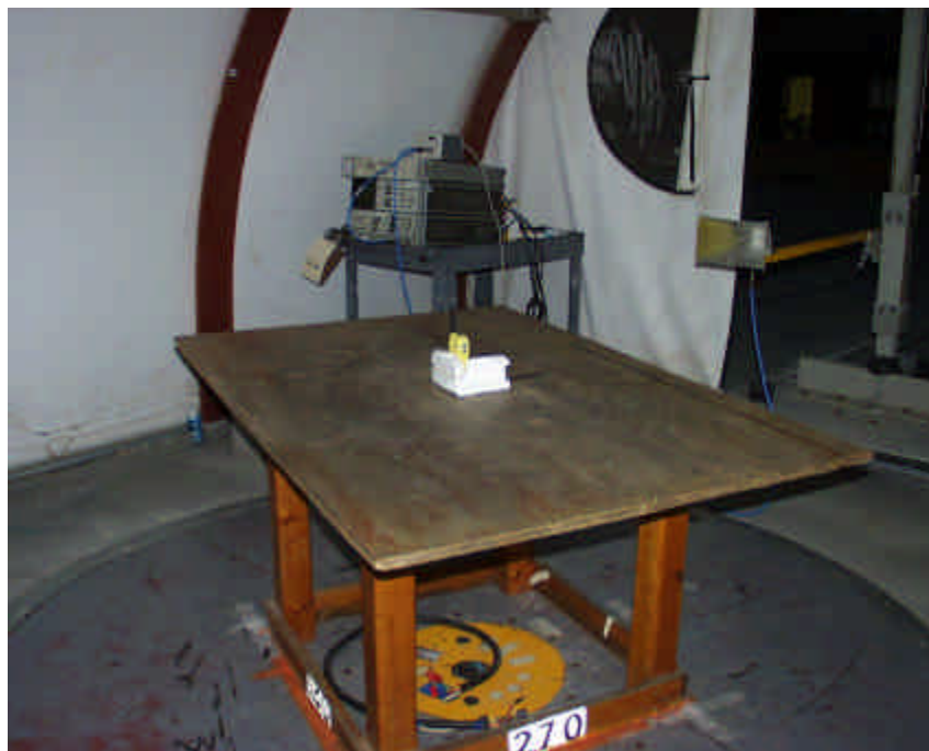
Radiated Emission above 1 GHz measurement setup
