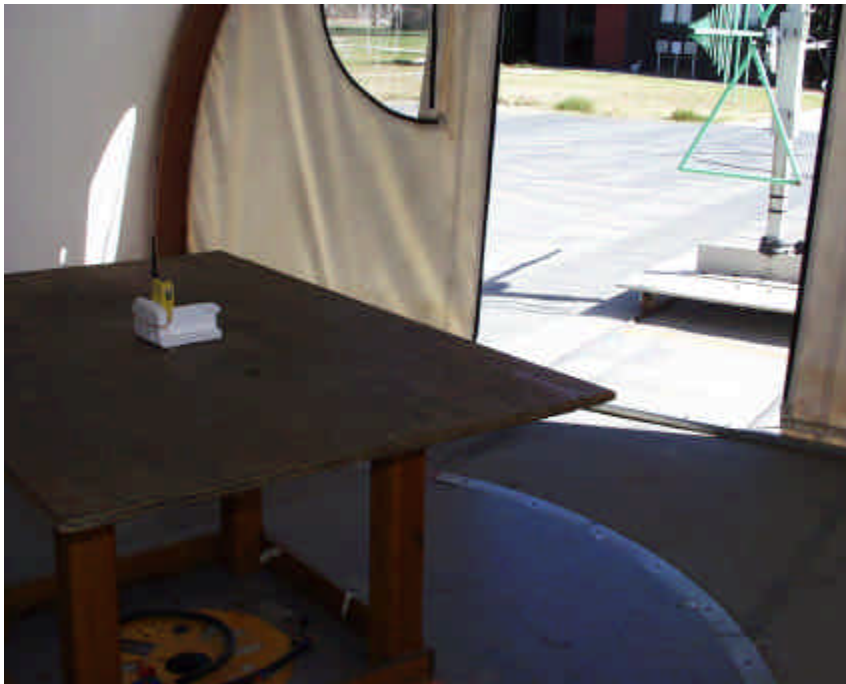
Radiated Emission Setup 30 – 1000 MHz
