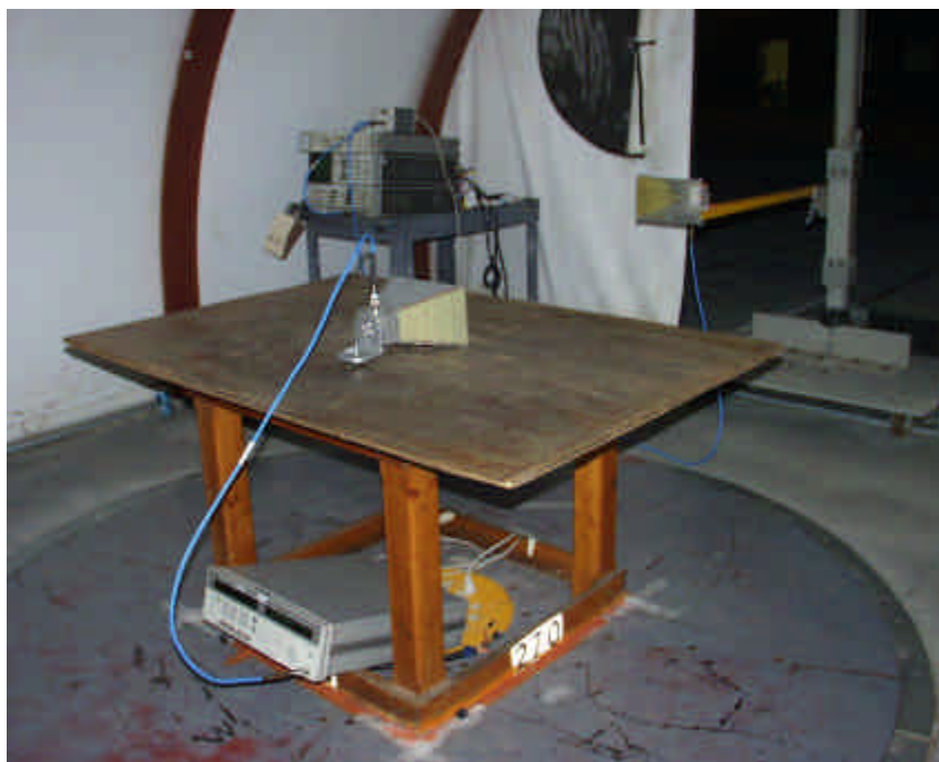
Above 1 GHz Substitution Method Setup
