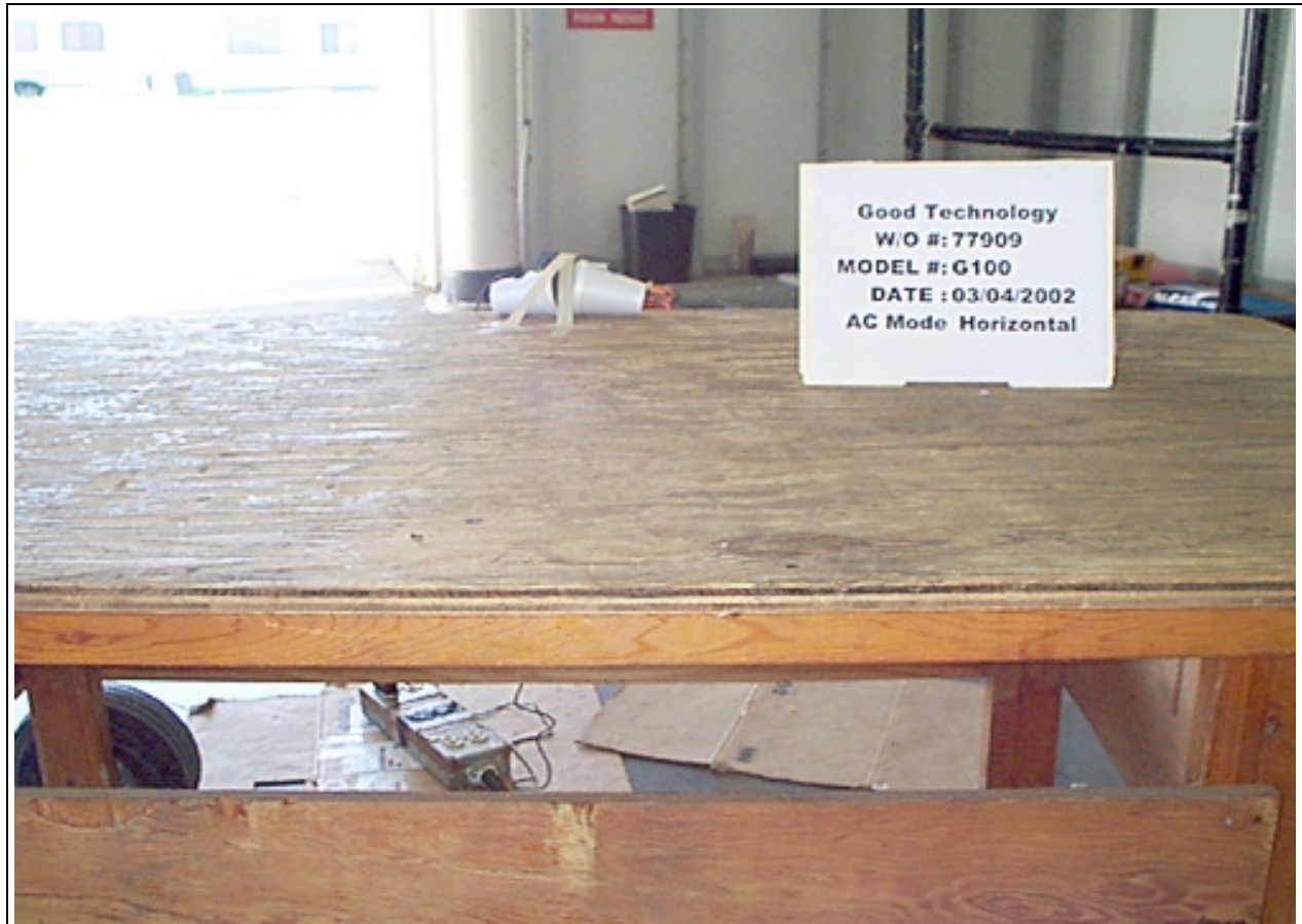
Radiated Emissions - Front View - AC Adapter Horizontal
