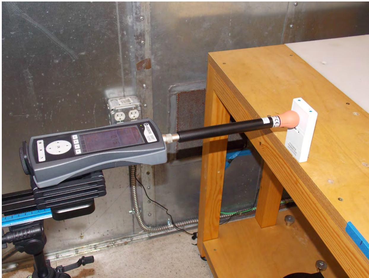
Testing Position at 20 mm All distances have the probe move away from the device
