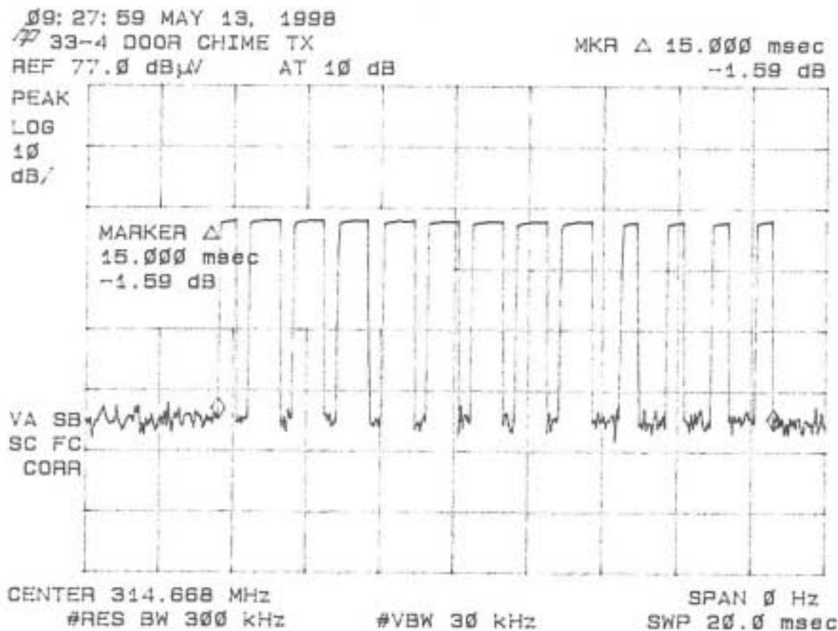
**Field Strength of Fundamental Emission (47 CFR 15.231b)**
