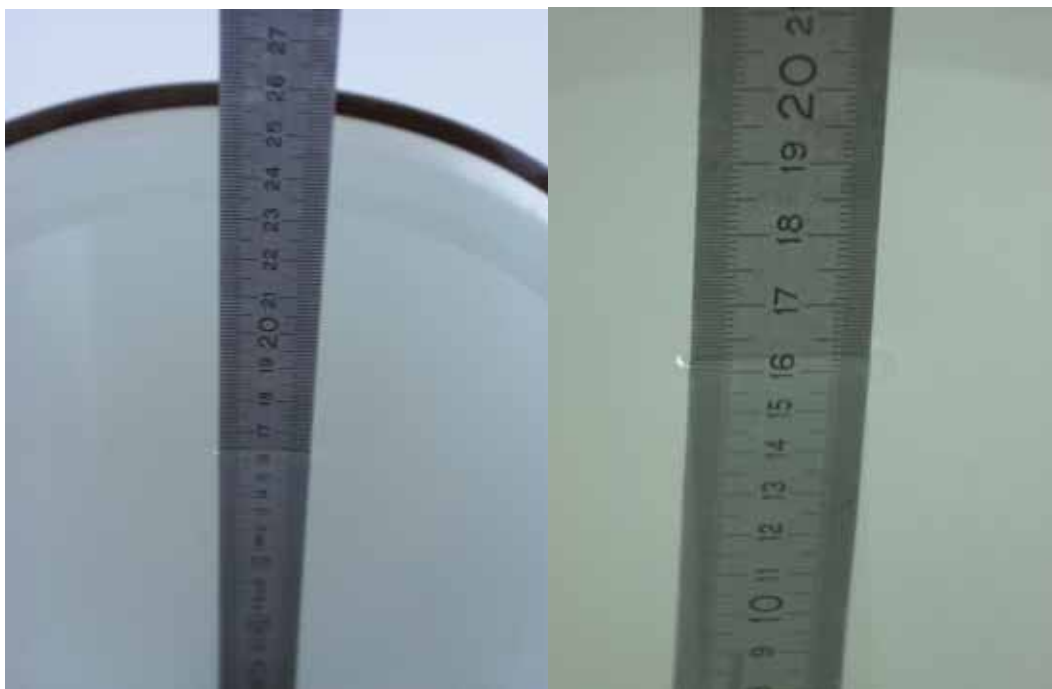
Fig. 39: Liquid depth for PCS 1900 Head and Body measurements.
