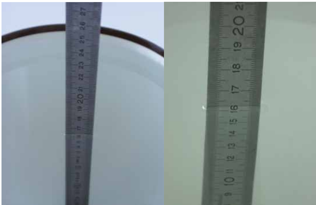
Fig. 29: Liquid depth for PCS 1900 Head and Body measurements.
