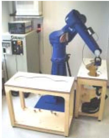
Fig. 6: The measurement set-up with two phantoms containing tissue simulating liquid.
