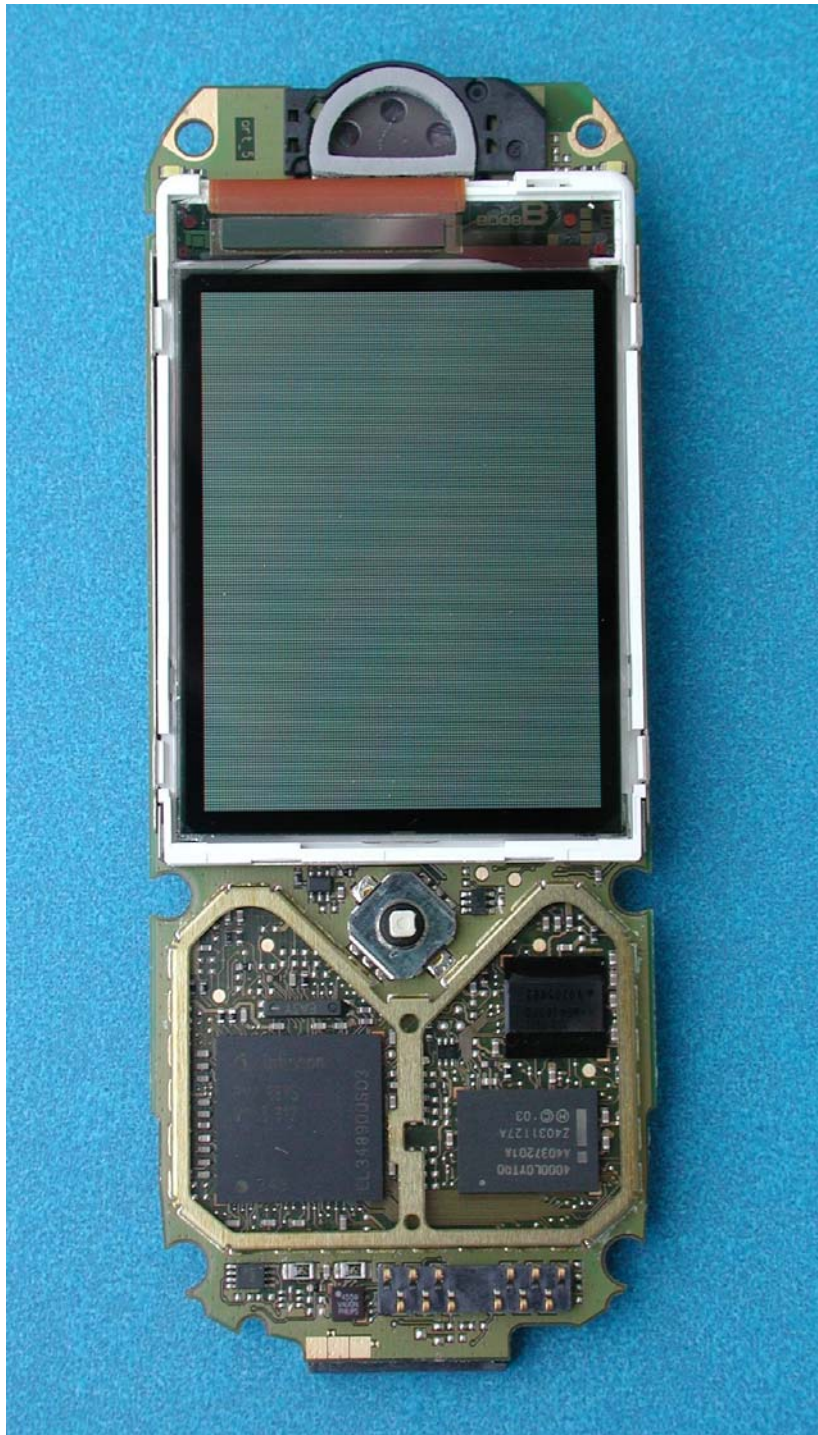
CX-65 PCB Front View Shields Removed
