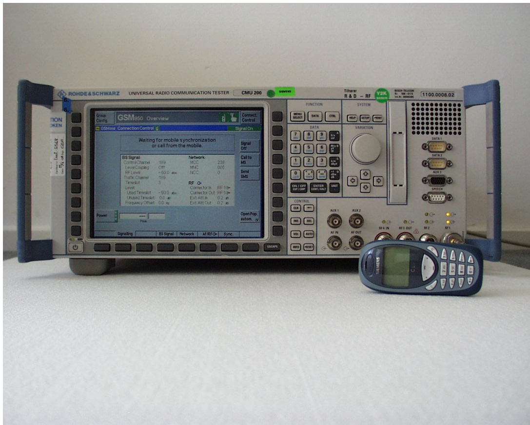
Figure 2: Set-up for conducted power measurement
