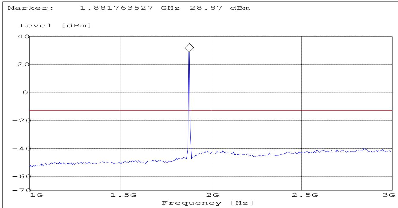
**RADIATED SPURIOUS EMISSIONS****Channel 661: 3GHz – 8GHz**
