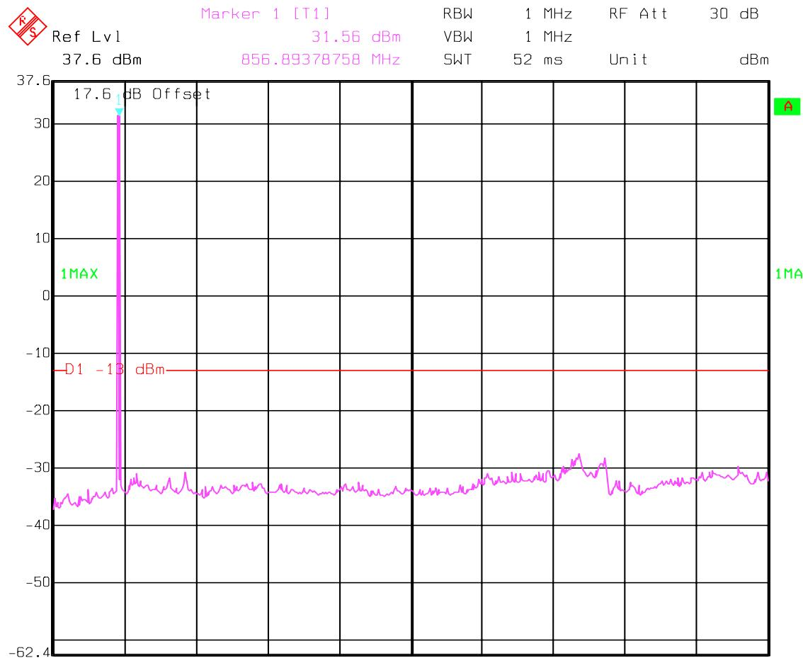
**CONDUCTED SPURIOUS EMISSIONS****Idle Mode (GSM-850)****30MHz – 9GHz**
