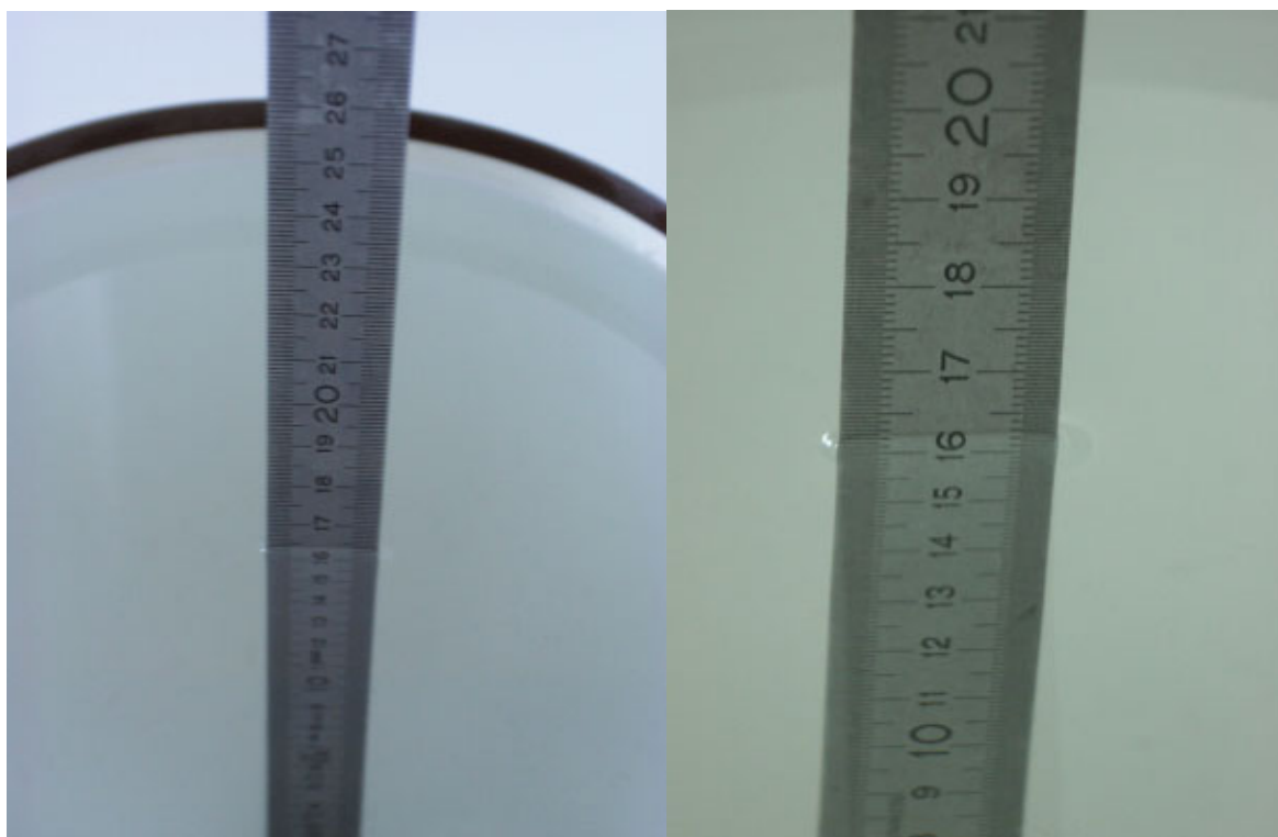
Fig. 63: Liquid depth for PCS 1900 Head and Body measurements.
