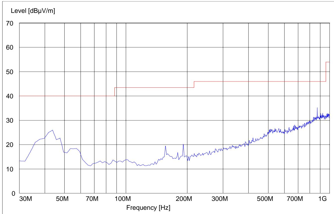
**RECEIVER RADIATED EMISSIONS****EUT in Idle Mode: 30MHz – 1GHz****Antenna: horizontal****SWEEP TABLE: "FCC 24 Spur 30M-1G"**
