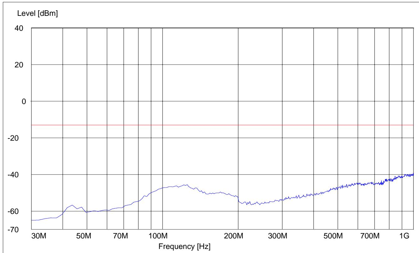
**RADIATED SPURIOUS EMISSIONS****Channel 512: 30MHz - 1GHz**
