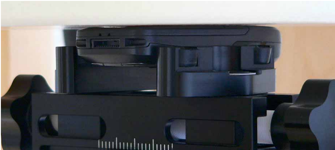
Fig. 29: Body worn configuration, GSM 1900 without accessory, antenna towards the phantom.
