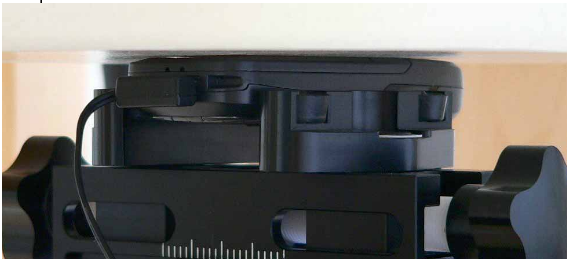
Fig. 30: Body worn configuration, GSM 1900, with headset, antenna towards the phantom.
