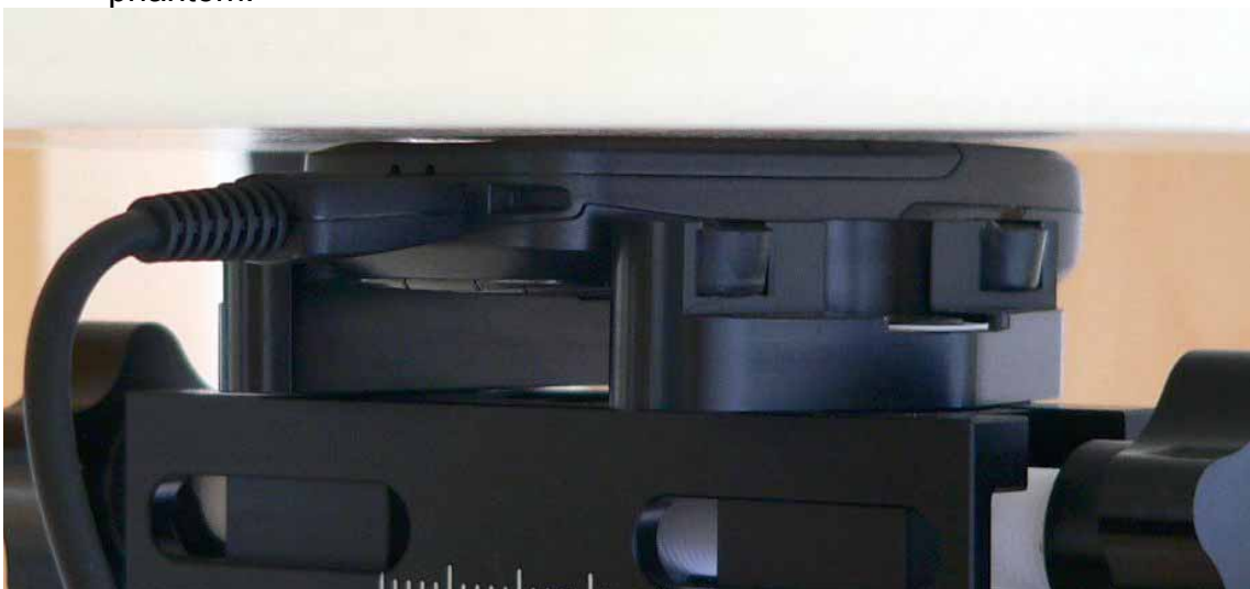
Fig. 31: Body worn configuration, GPRS 1900 (Class 8) with data cable, antenna towards the phantom.
