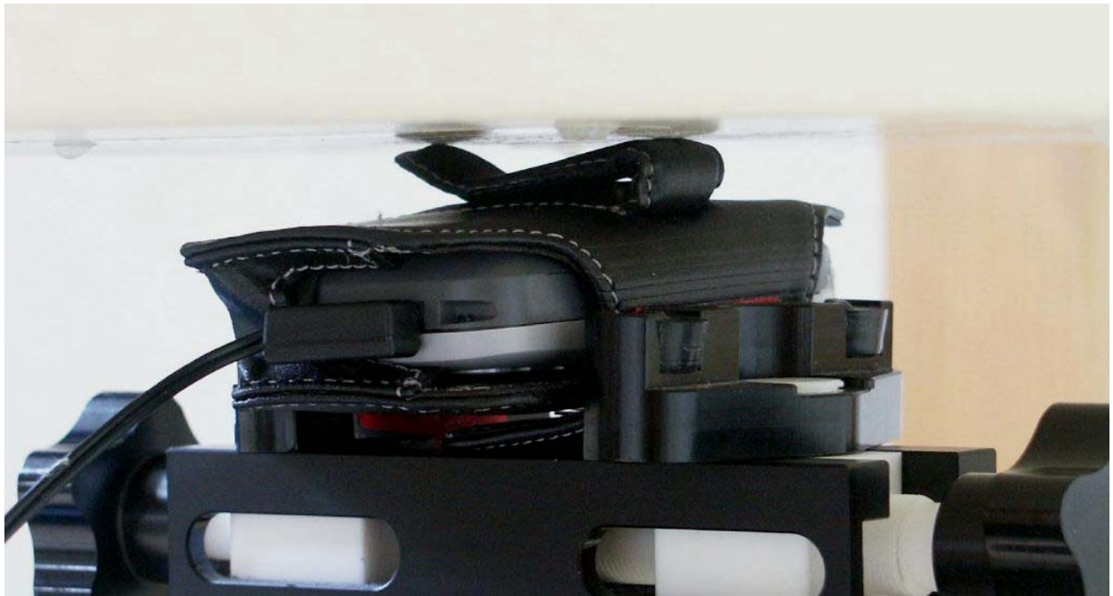
Fig. 21: Body worn configuration, GSM with headset and FCL600, antenna towards the phantom (13 mm distance).
