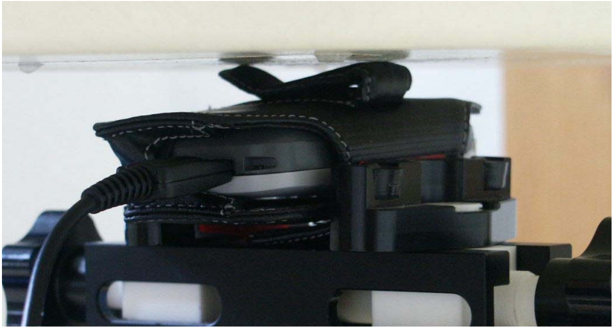
Fig. 22: Body worn configuration, GPRS Class 8 with data cable and FCL600, antenna towards the phantom (13 mm distance).
