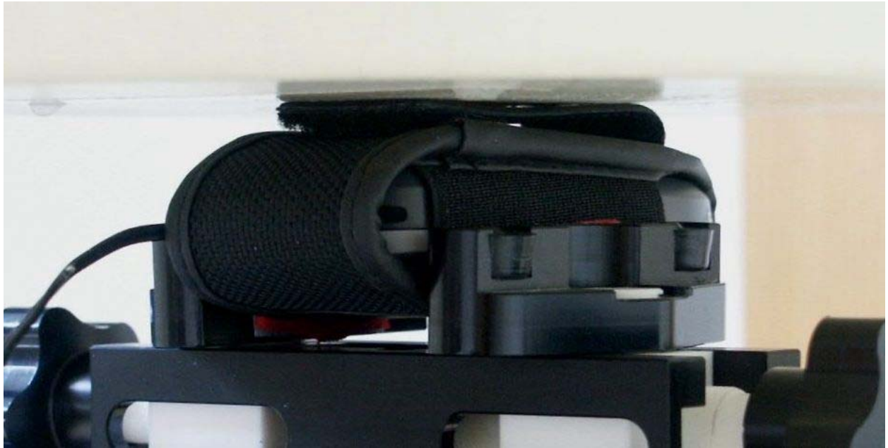
Fig. 20: Body worn configuration, GSM with headset and FCT650, antenna towards the phantom (10 mm distance).
