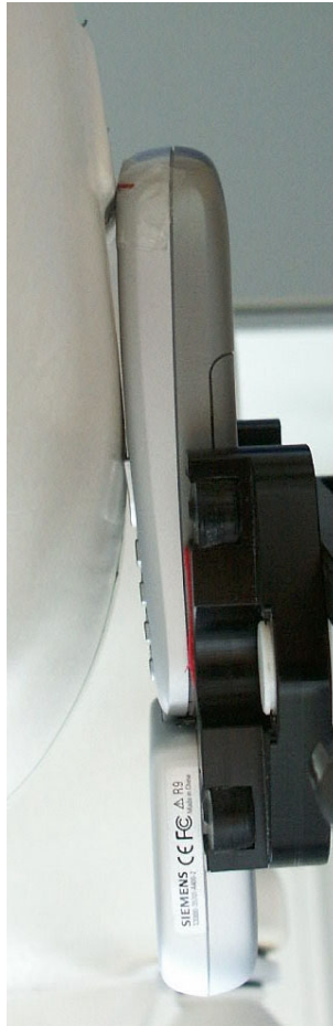
Fig. 22: Cheek position, left side with cam.
