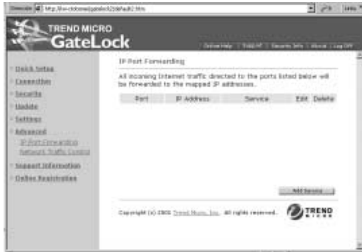
FIGURE 3-25. Use the IP Port Forwarding screen to control access to your servers
