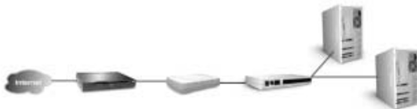
FIGURE 2-3. Connecting Multiple PCs to the Internet with GateLock
