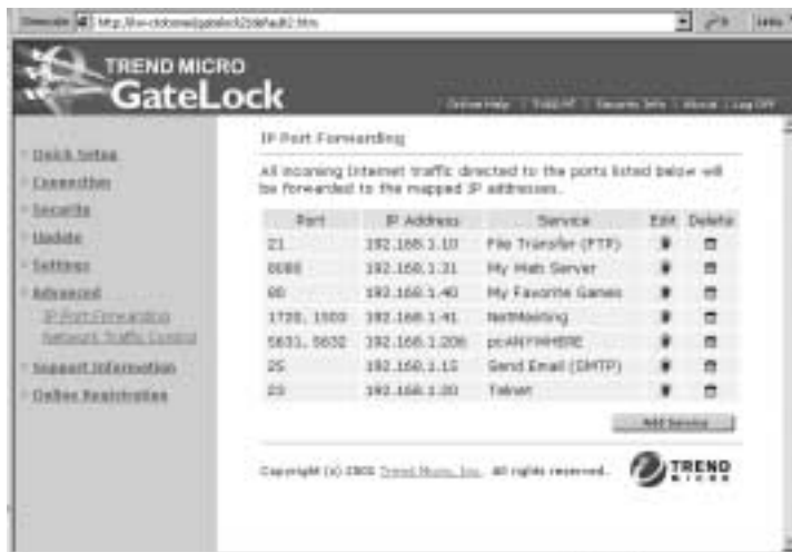
FIGURE 3-27. What the IP Port Forwarding screen looks like after Internet services have been added
