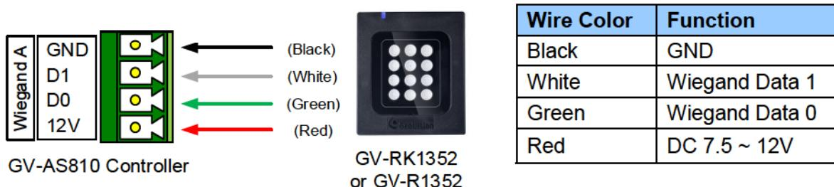
**Note:** Connection through Wiegand interface is not supported for GV-AS1010.
