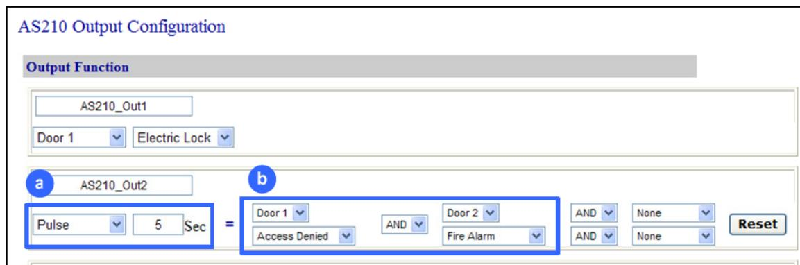
2. Find the output wired to the beeper or LED and specify up to 2 alarm conditions to set off the beeper or LED.
