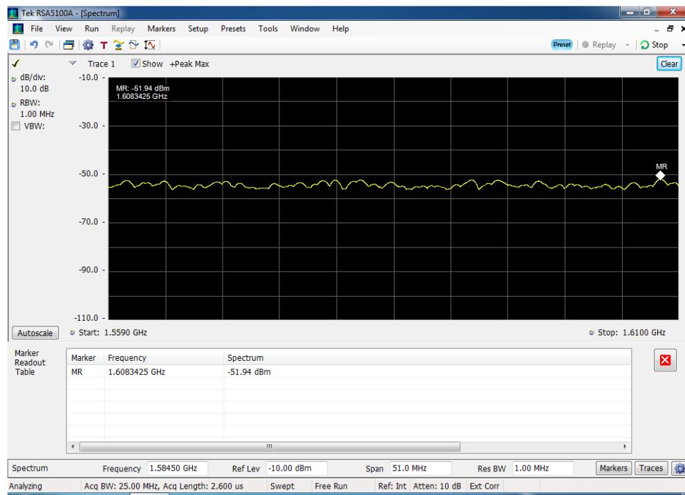
Cond Spur \_UL\_B13\_776 - 787 MHz\_RBW=700 Hz\_1559 - 1610 MHz\_S3 to Common D1
