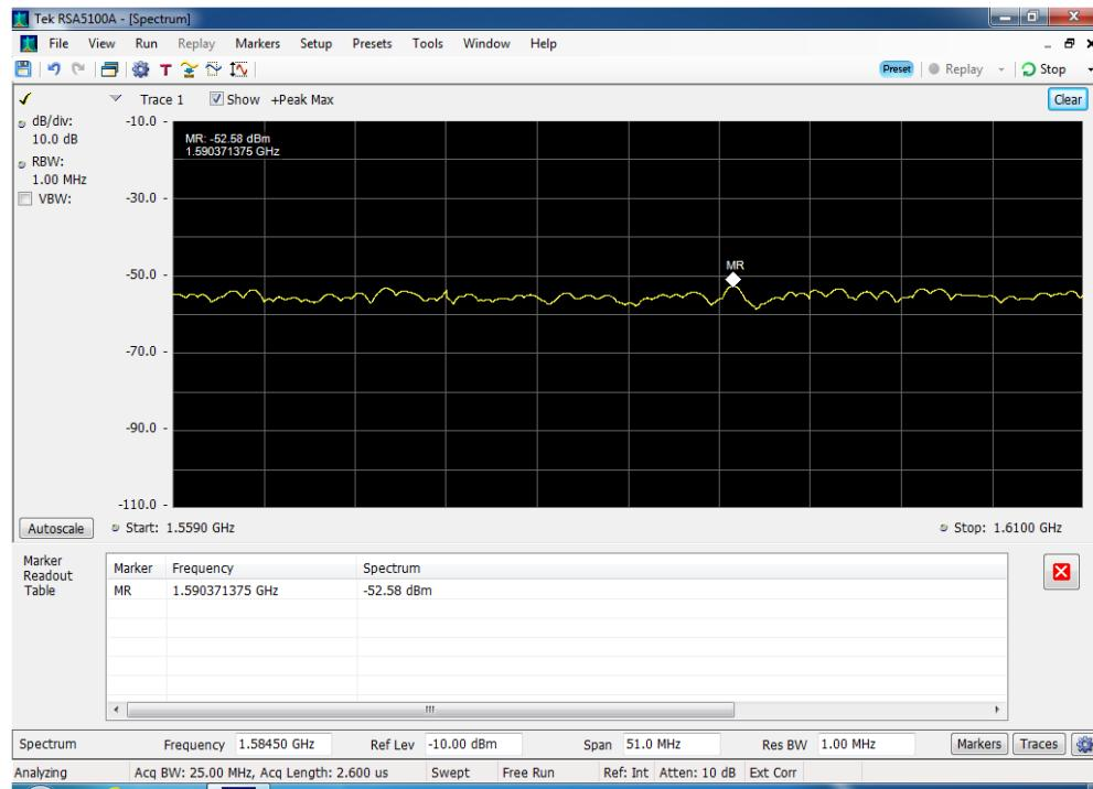
Cond Spur \_DL\_B13\_746 - 757 MHz\_RBW=1 MHz\_1559 - 1610 MHz\_D3 Common to S2
