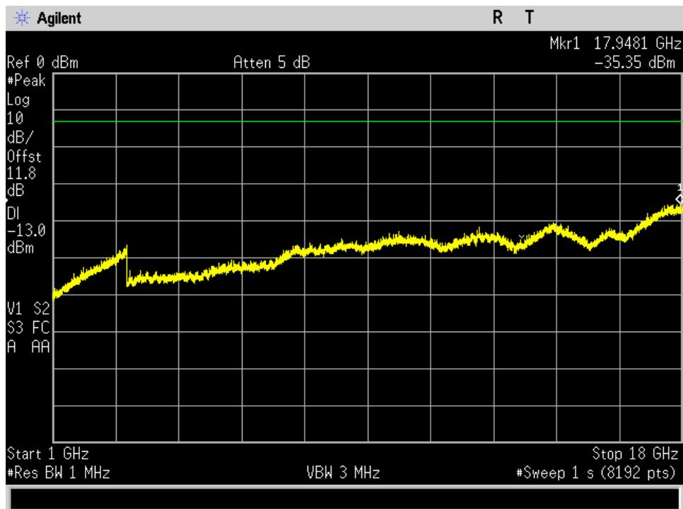
**Radiated Spurious\_DL\_728 - 746 MHz\_30 - 1000 MHz**
