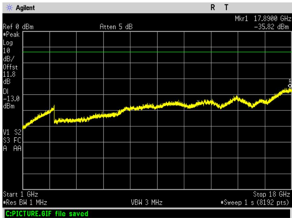
**Radiated Spurious\_DL\_746 - 757 MHz\_30 - 1000 MHz**
