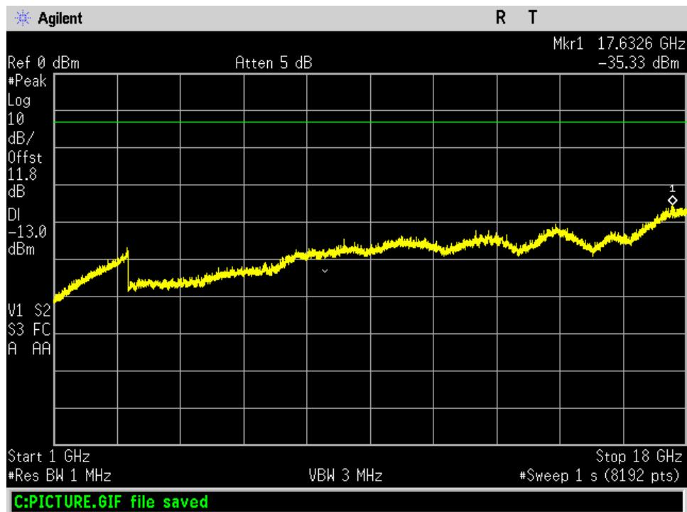
**Radiated Spurious\_UL\_1710 - 1755 MHz\_30 - 1000 MHz**
