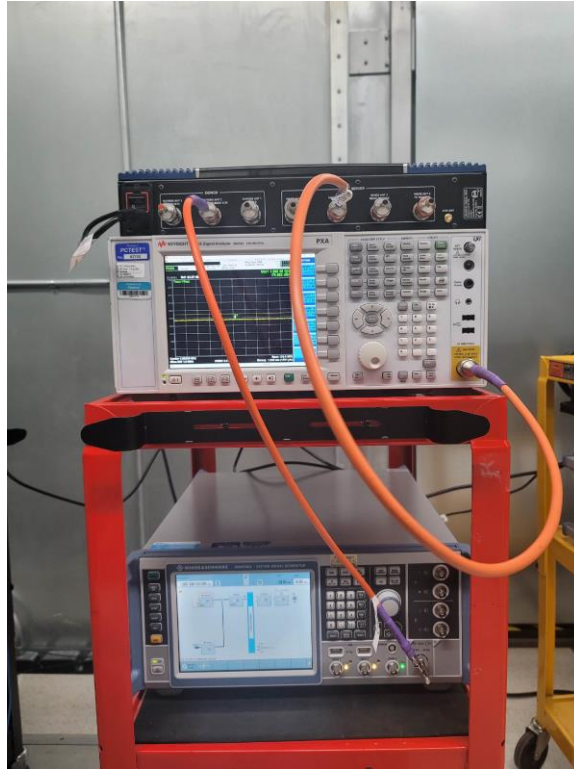
Figure 7. Downlink test configuration in EUT test mode
