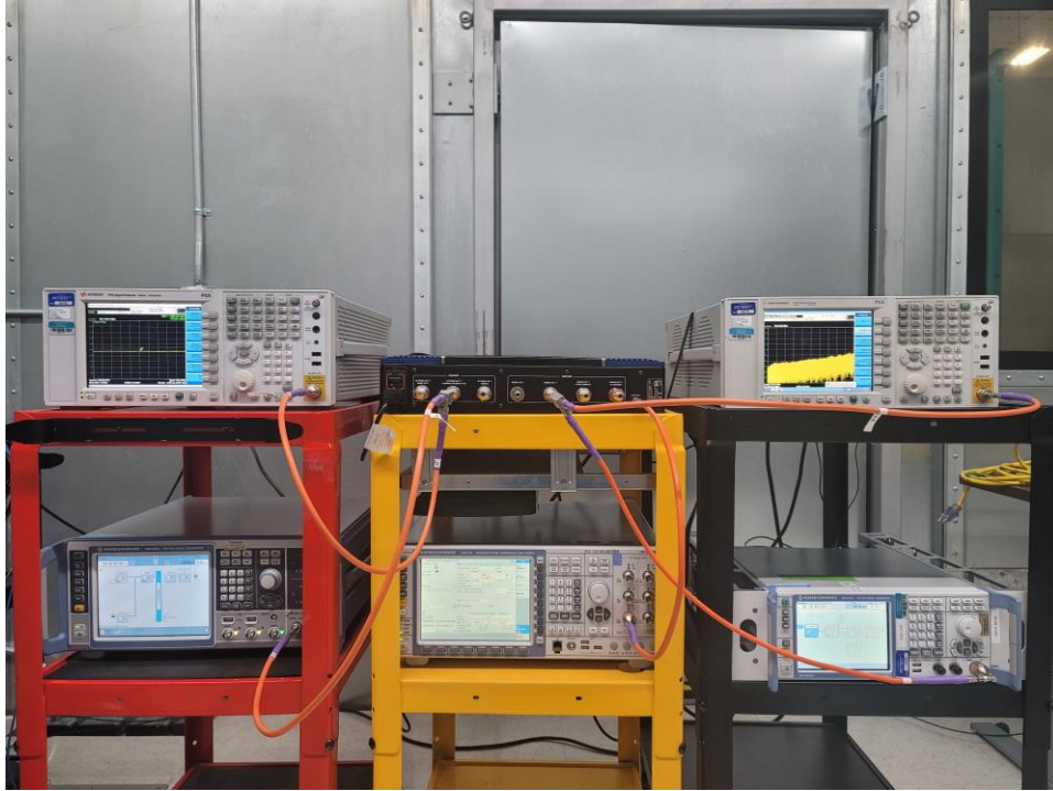
Figure 5. Test configuration in EUT normal operational mode
