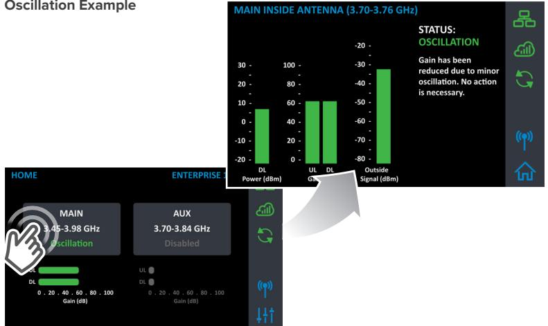
**Note:** If the reduced gain due to oscillation is greater or equal to 60dB, the condition will be displayed as Green and no action is necessary.
