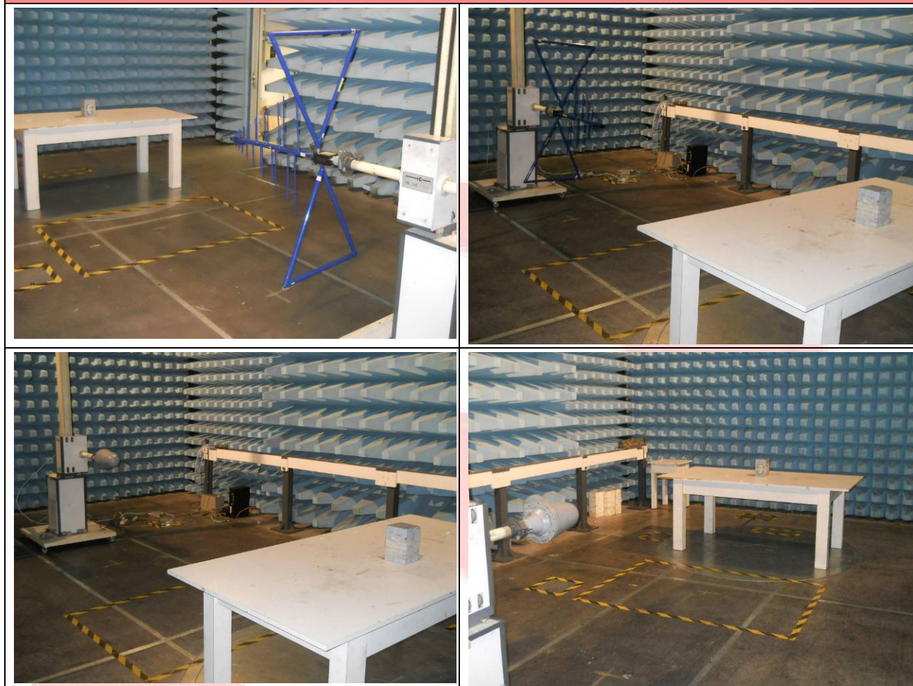
PHOTO N° 2 –RADIATED EMISSION SETUP
