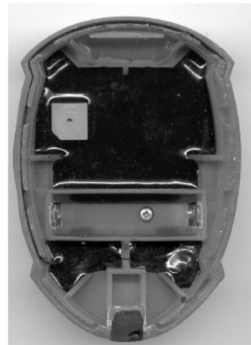
11.7 Galeo - rear view with circuit resinated
