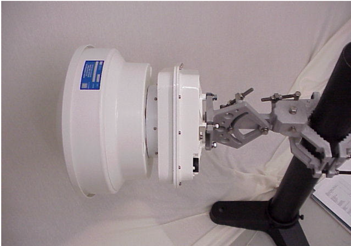
3261-0000, 3264-0000 Top Level with antenna, mounting bracket, mounted on pole
