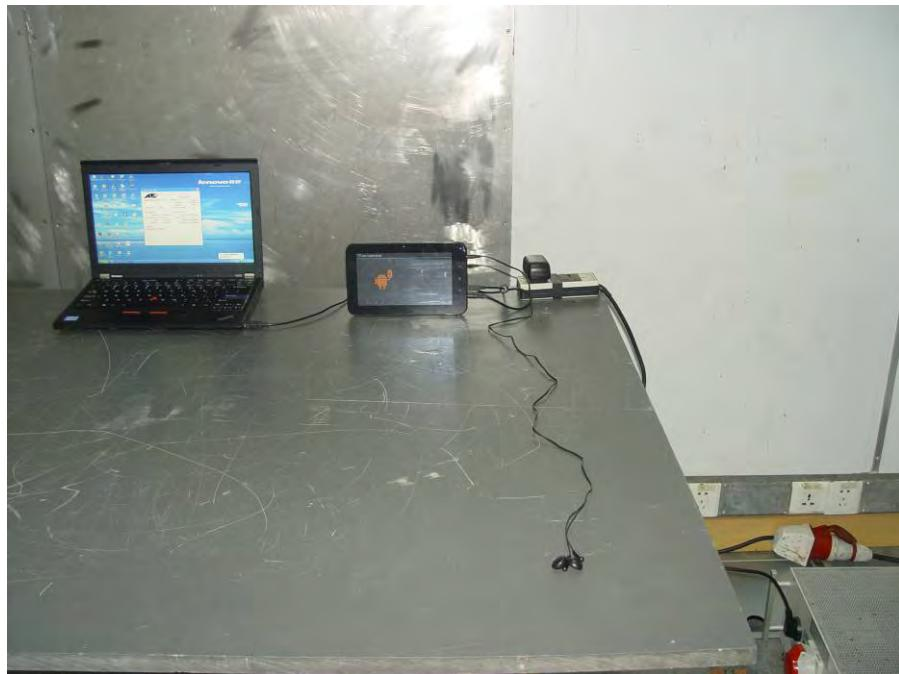
Radiated emission up to 1G (Transfer data Mode)
