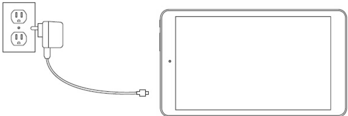
Plug the charger into a power outlet. Keep the battery on charge for 6 to 8 hours to make sure that it is fully charged.
