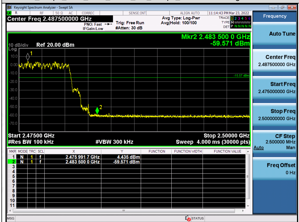
Test_Graph_EDR_HOP_ANT1_NA_3Mbps_Higher Band Edge Emissions
