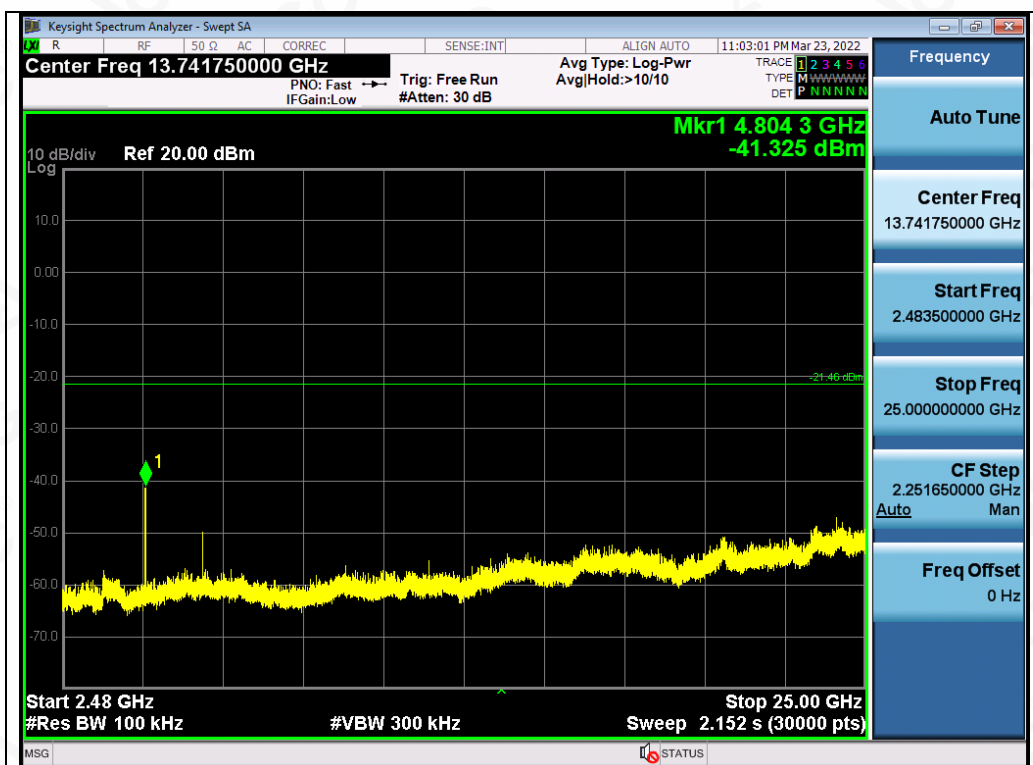
Test_Graph_EDR_ANT1_2402_3Mbps_Higher Band Emissions
