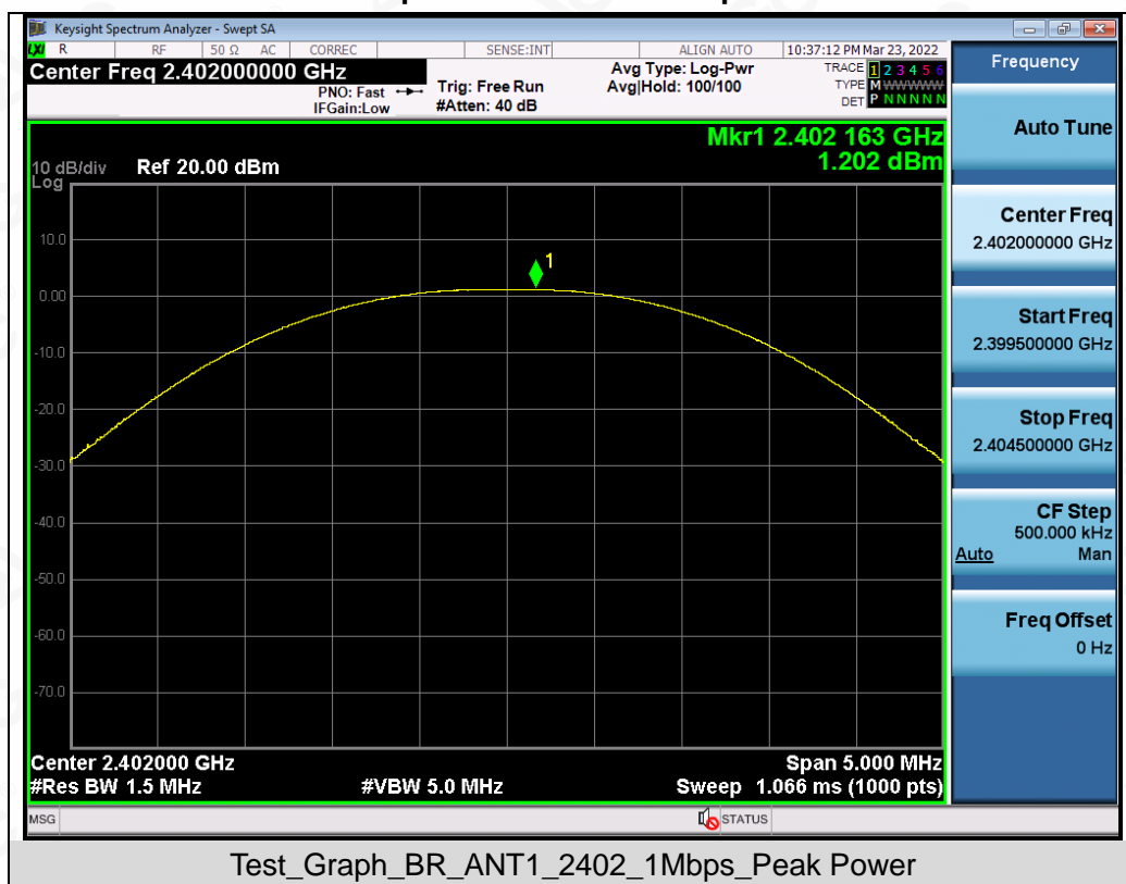
Test Graphs of Conducted Output Power
