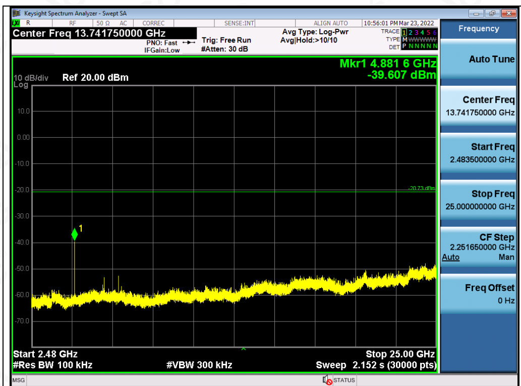
Test_Graph_EDR_ANT1_2441_2Mbps_Higher Band Emissions
